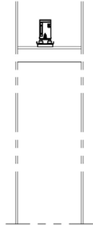
KTR 953 RECEIVER / EXCITER INSTALLATION VIEW LOOKING OUTBD ON WARDROBE AVIONICS RACK
