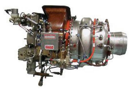
The modification involves the removal of the APU Starter/Generator and the APU engine. The remaining APU system components such as the FADEC and APU Fuel Pump are disabled.
