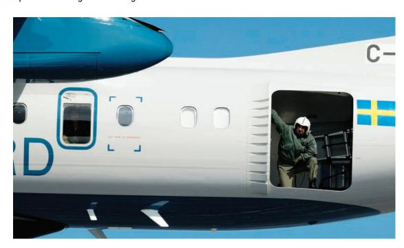
The AOD utilizes the existing inward-opening, plug-type OEM cargo door, which is modified to add an internal handle for opening and closing the door. Other modifications include a secure attachment point for the safety line for two crew members, non-slip flooring and a fuselage mounted air deflector.
