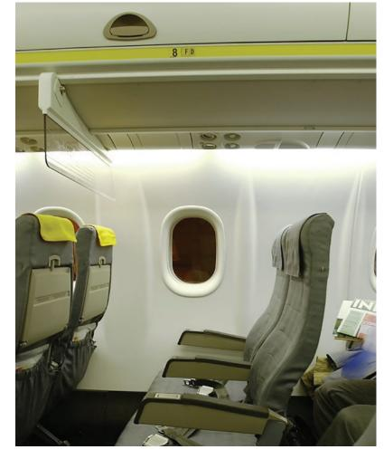
back of any row, except immediately forward of the mid-cabin emergency exits. It can be installed at the last seat row, immediately forward of the aft bulkhead, for storage when dual class service is not required.
