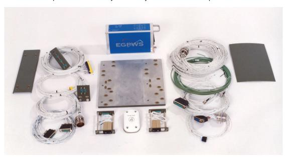
The existing MK II GPWS system components are removed or deactivated. Existing wiring is re-terminated and new wiring is added. A new mounting tray is installed in the previous MK II location and a GPS antenna is installed on the upper fuselage. Annunciator sets are installed on the pilot's and copilot's flight panels. A temperature probe is installed on the lower fuselage on Series 100 aircraft only.
