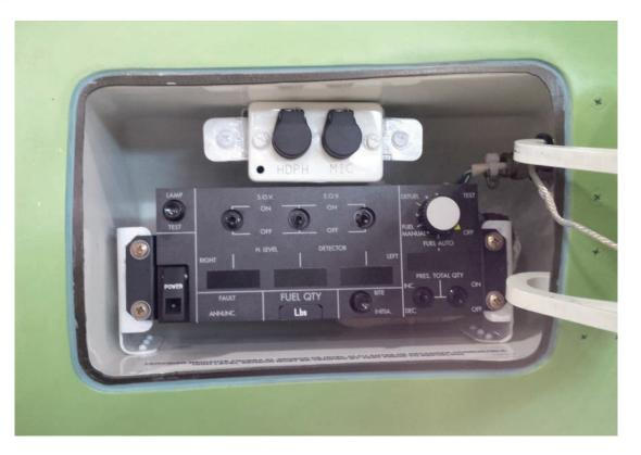
On the CRJ 100/200, the customer removes the existing refuel/defuel control panel from the aircraft and sends it to FIELD AVIATION for conversion to the required units. The converted refuel/defuel control panel is sent back to the customer for re-installation in the aircraft. On the CRJ700, a replacement refuel/defuel panel is required.
